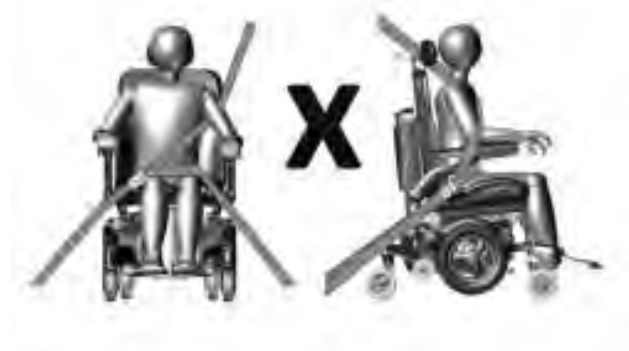
Figure 5.6 – incorrect positioning of three-point occupant restraint
