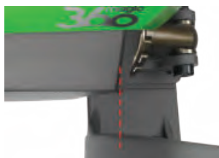
Figure 4.7 – Shock absorber adjustment
