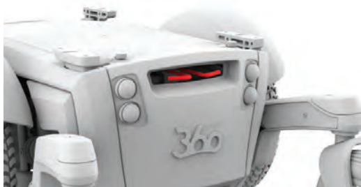
Figure 4.4a Magic 360 brake levers engaged
