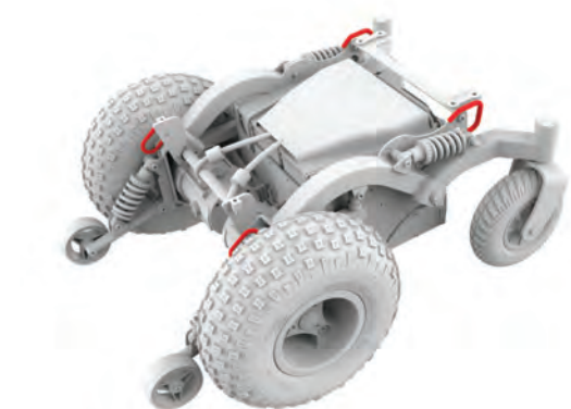
Figure 5.2c Frontier V4 lifting points
