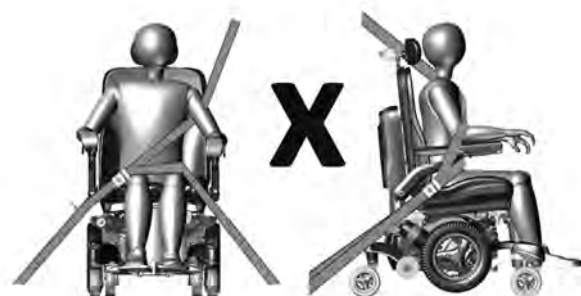
Figure 5.6 – incorrect positioning of three-point occupant restraint
