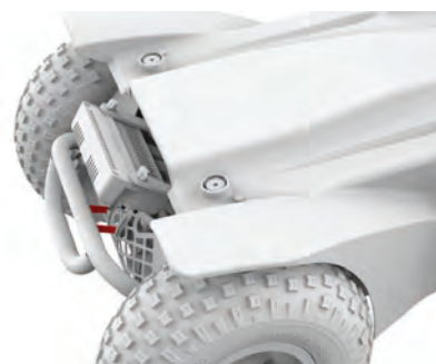
Figure 4.6b X8 brake levers released
