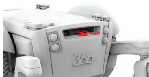
Figure 4.4b Magic 360 brake levers released
