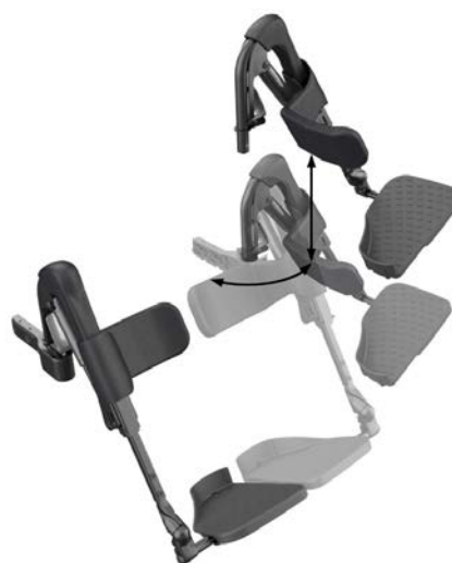
Figure 4.2c Swingaway Legrest showing removal action
